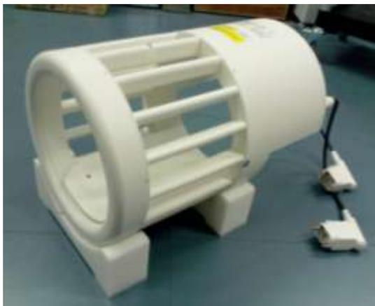
Dual-resonance  $^1\text{H}/^7\text{Li}$  RF coil
