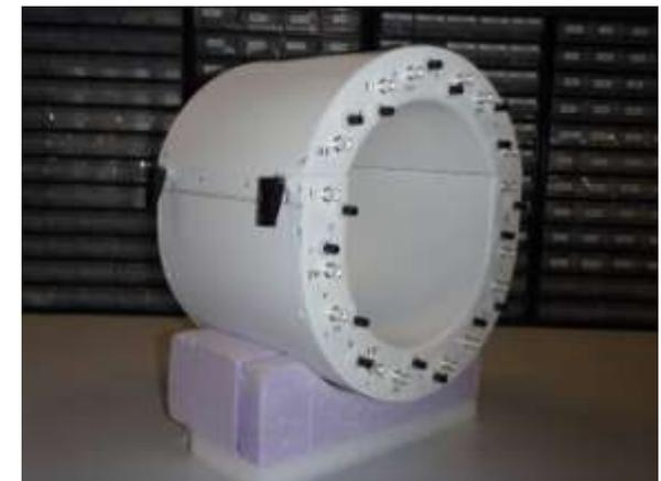
Dual-resonance  $^1\text{H}/^{31}\text{P}$  RF coil (from Resonance Research Inc)
