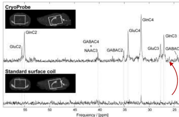
Despite its limitation at UHF to preclinical MRI, cryogenic RF coils holds the promise of a large increase in NMR sensitivity for X-MRI.
